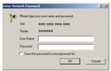
**3.** Enter a valid user name and password according to the Login mode selected in step 2, and click [OK] to log in to the camera.
